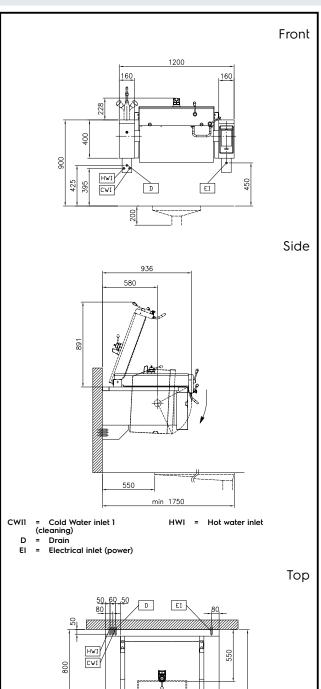
**Electric** Supply voltage: 400 V/3N ph/50/60 Hz 15.5 kW **Total Watts:** Installation:
